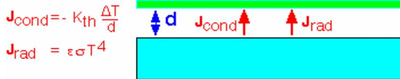
Here we show calculated fluxes in the simple case where the upper (cool) surface is a perfect black absorber, held at room temperature.
