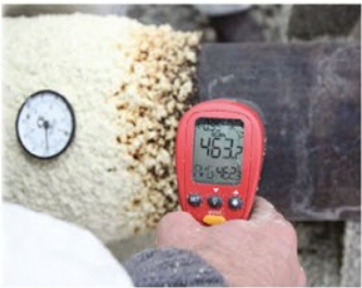
Before HPC® Coating application 463°C (865.4°F).
