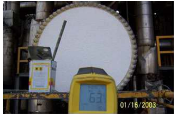
Surface temperature after applications, reduced by 68%
