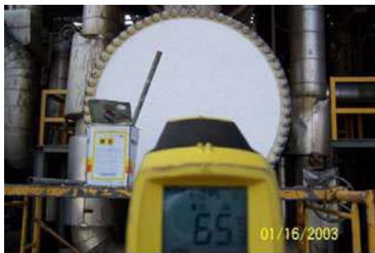
Surface temperature after applications, reduced by 68%
