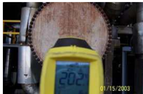
Surface temperature measurement before coatings
