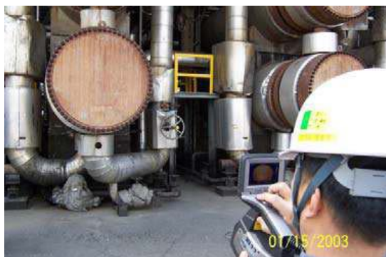
Surface temperature measurement before coatings
