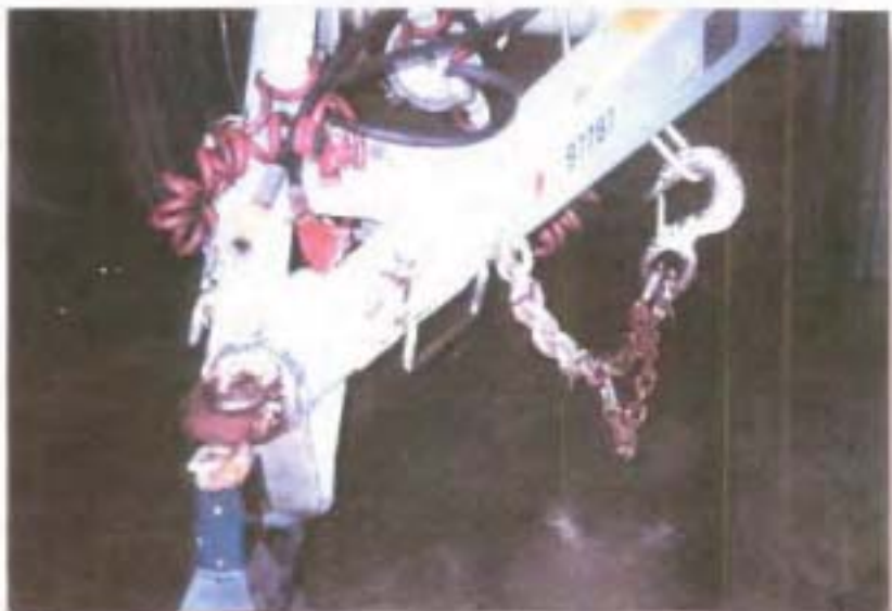
TRUCK DOLLY BEFORE COATING WITH RUST GRIP NOTE THE CORROSION THAT PREVIOUSLY WOULD TAKE HOURS TO GRIND TO WHITE METAL.
