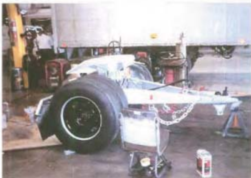
TRUCK DOLLY BEING COATED WITH RUST GRIP IN LESS THAN 20 MINUTES USING A PLASTIC SPRAY BOTTLE. RUST GRIP WAS APPLIED DIRECTLY OVER THE RUST.
